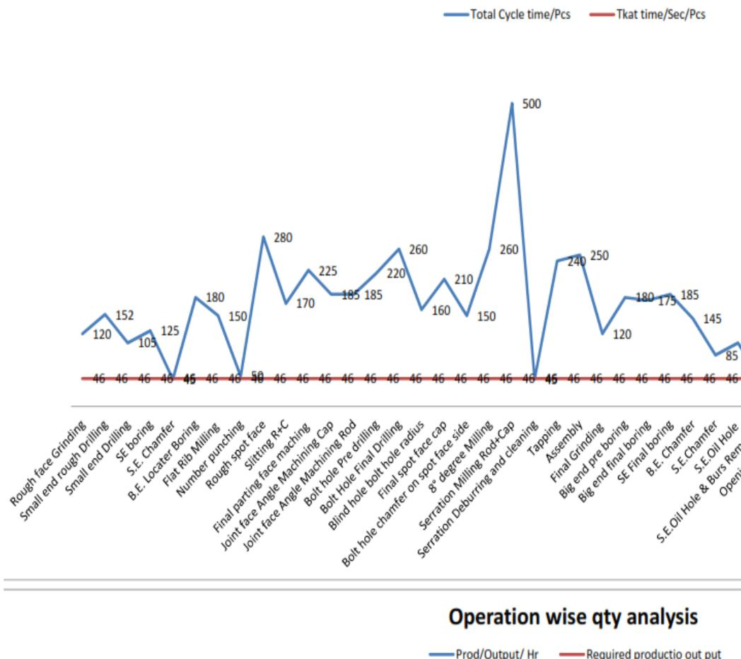
Fig. 5. Operation wise quantity analysis (Before)
