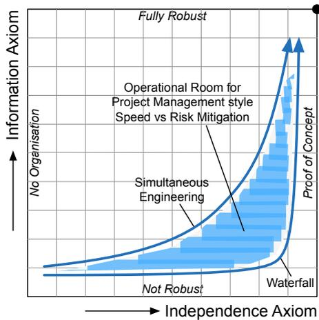
**Fig. 3.** Depending on the nature of the project, a different strategy may be followed. The right lower curve would represent a waterfall management approach, while the upper would represent the path in case of a simultaneous engineering strategy
