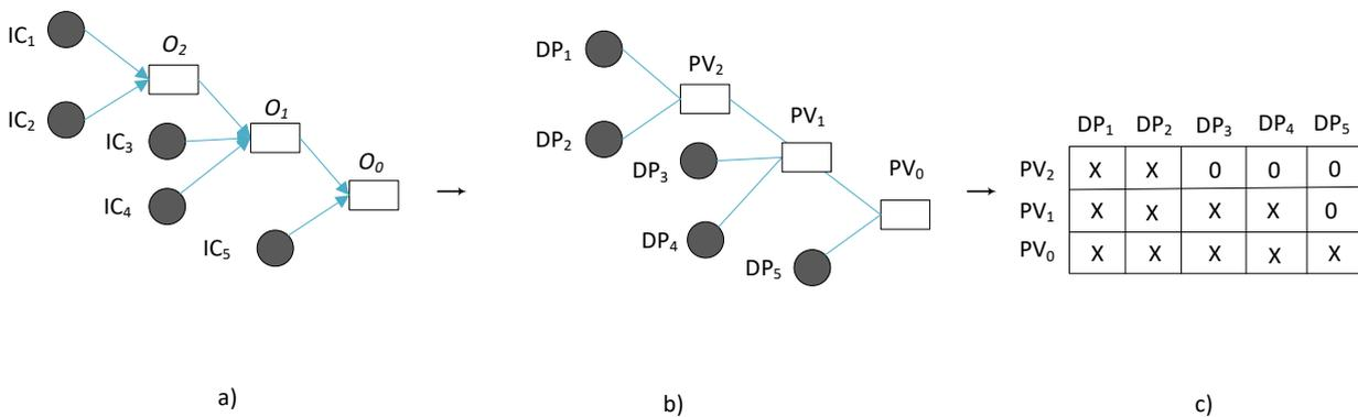
**Fig. 8.** a) Initial model of assembly process structure; b) Converted model of assembly process structure; c) Transformation of the converted process structure into DM.
