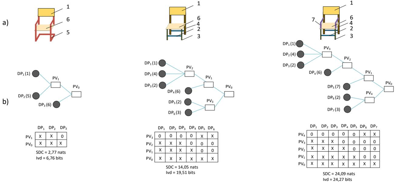
**Fig. 11.** a) Design variants of customized chair; b) Related process models of assembly operations with DMs.
