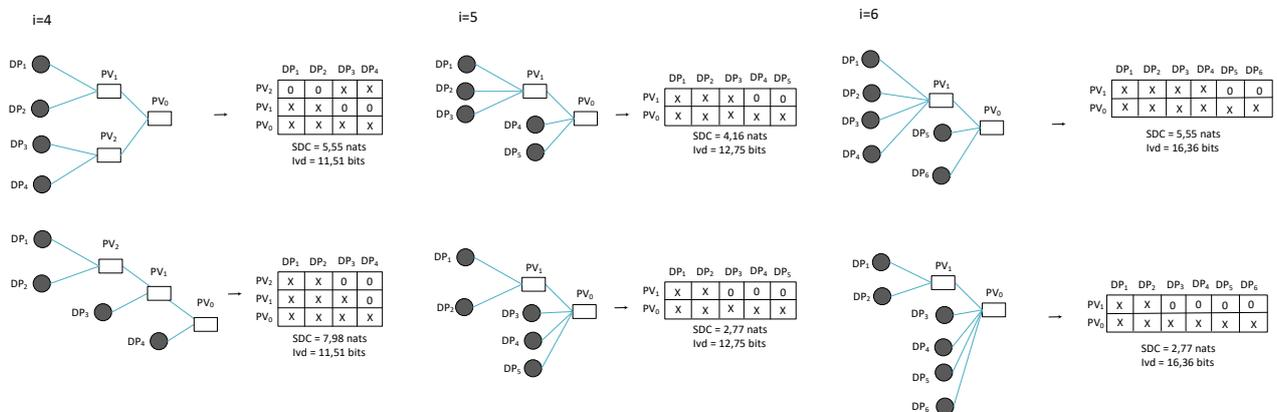
**Fig. 12.** An examples of process structures containing four, five and six assembly ICs with SDC and Ivd values.
