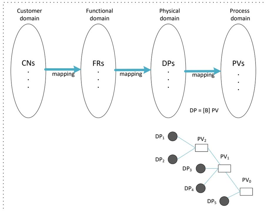
Fig. 9. The relation between input assembly components and process nodes in context of four domains of the design world.
