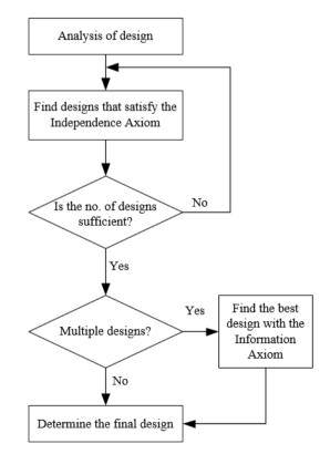
Fig. 1. Flowchart of the application of Axiomatic Design [11]
