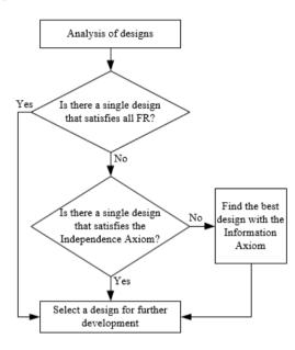
Fig. 2. Modified flowchart of the application of Axiomatic Design
