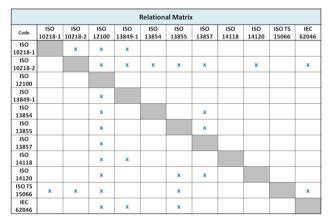
Fig. 3. Relational Matrix about main safety of machinery standards for robotic-cell applications.
