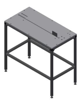
Figure 10. The final concept for the linear actuator integrated in the table. The fin transfers the motion to the top of the table, all active elements can be placed below the level where the boxes are handled.
