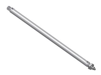
**Figure 9.** Festo DSNU [7] pneumatic cylinder in 500 mm length with 25 mm piston diameter. The cylinder is shown in the retracted state. When the piston is extended, the overall length almost doubles.
