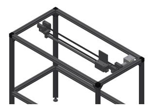
**Figure 11.** The table top has been removed and the rails, the stepper motor, the timing belt, the sprockets and various support brackets are revealed.
