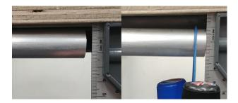
Fig. 15. Deflection of a 50 cm long,  $20 \times 1$  mm aluminum tube. 1 kg mass at end.
