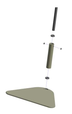
Fig. 10. Assembly presentation of the bearing block.
