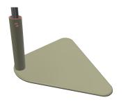
Fig. 9. The bottom plate with the bearing block.
