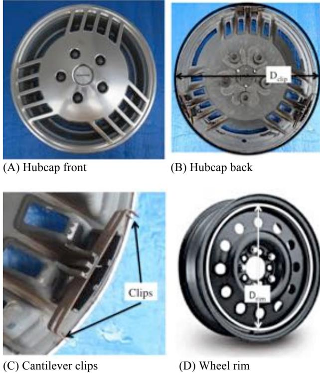
Fig. 1. Attachment of hubcap to wheel rim
