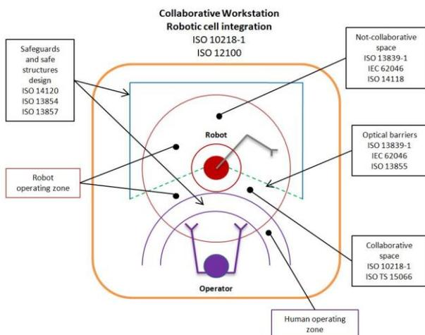
Fig. 9. New design of the collaborative assembly workplace.
